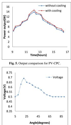
Fig. 6. Optimum trough angle for Single mirror concentrator.
