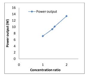
**Fig. 8.** Variation of Power output with concentration ratio.
