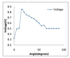
**Fig. 7.** Optimum trough angle for V-trough concentrator.
