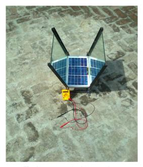
Fig. 1. PV-V-trough without cooling.
