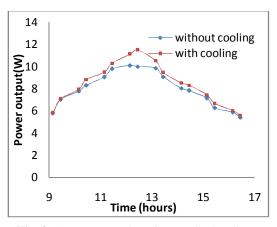
Fig. 3. Output comparison for PV-single mirror concentrator.
