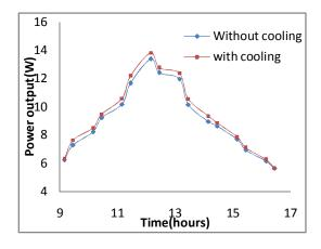
Fig. 4. Output comparison for PV-V-trough concentrator.
